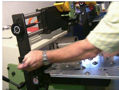
6. Fix the device stop in place with a screw
